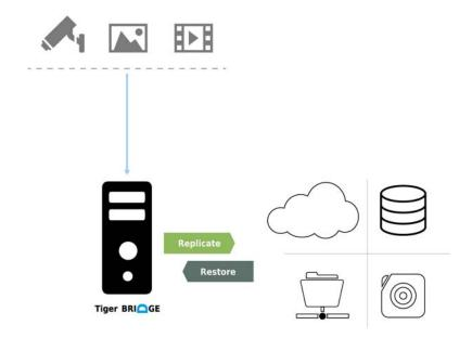
**data replication** — Tiger Bridge copies a file from the source to the target. Automatic replication is performed based on user defined criteria. You can also manually replicate a file or a
