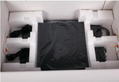
**7.** Take out the two foam chassis protectors and with two people holding the appliance at each side, take it out of the box and place it on a surface, ensuring that the system remains stable.
