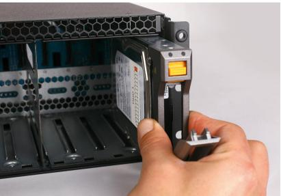
Tbox Assembly Guide Site Installation: Installing the Drives
