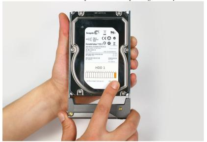
**4.** Slide the drive carrier into the corresponding slot until the latch makes contact with the enclosure.
