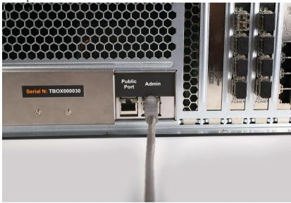
2. Plug other end of the network cable in the LAN port of the computer, from which you want to perform initial connectivity setup.
