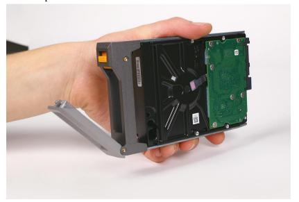
Tbox Assembly Guide Site Installation: Installing the Drives
