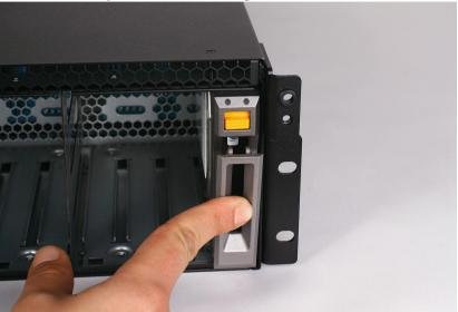
**6.** To check that the drive carrier is properly installed and makes full contact with the drive bay, try to pull it out without unlocking the latch.
