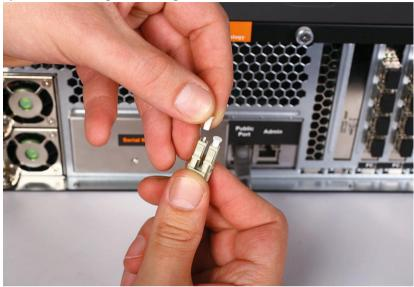
**3.** Plug one end of the FC cable into the SFP socket of the appliance port.
