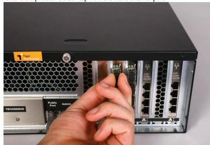
Tbox Assembly Guide Site Installation: Cabling Tbox
