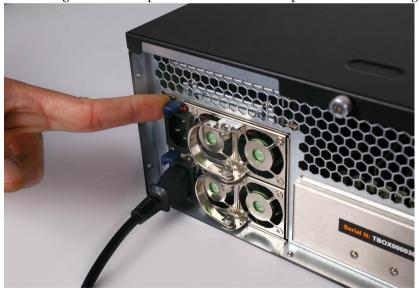
**4.** While pressing the button, pull the lever at a 90-degrees angle and slide out the unit from the appliance.
