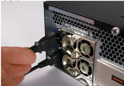
**3.** With the finger of one hand push the side button of the power module to the right.
