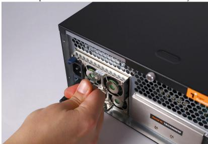
**6.** Push back the lever of the power module to lock it.
