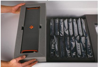
**4.** Take out the foam case with the spare RAID drive, the Tbox System Restore USB Flash Drive and the instructions CD.
