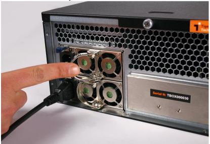
**7.** Plug the power cable in the module's socket.
