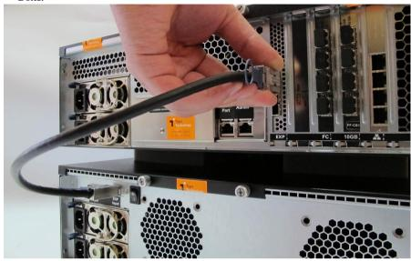
Should you decide to connect more expansion chassis (more than two with Tiger Box or more than one with Tiger Box1), you should plug the other end of the SAS cable in the Output port of one of the already connected expansion chassis.
