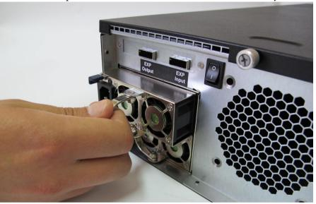
**6.** Push back the lever of the power module to lock it.
