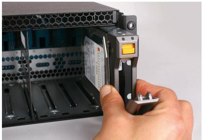
**5.** Push the latch up to finish sliding the drive carrier into the drive bay. To ensure that the latch is locked, you must hear a clicking sound.
