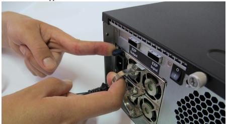
**5.** Insert the new power module and hear the side button click into the bay.
