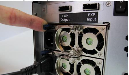
**4.** While pressing the button, pull the lever at a 90-degrees angle and slide out the unit from the appliance.
