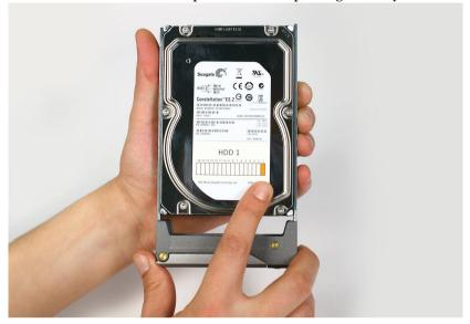
**4.** Slide the drive carrier into the corresponding slot until the latch makes contact with the enclosure.
