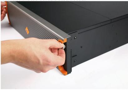
**2.** Gently pull away the bezel from the front panel of the expansion chassis.
