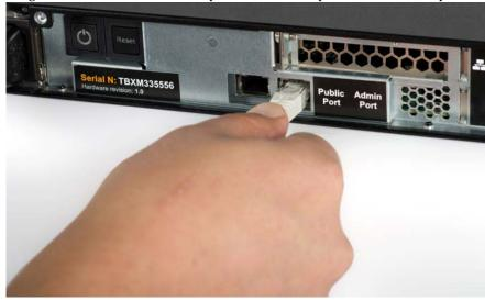
${\bf 2.}$  Plug other end of the network cable in the LAN port of the computer.
