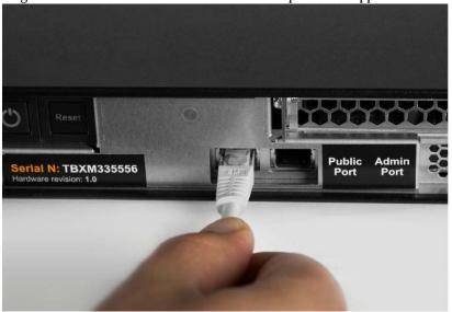
**6.** Plug other end of the network cable in the port of the Ethernet switch that interconnects computers on the network.
