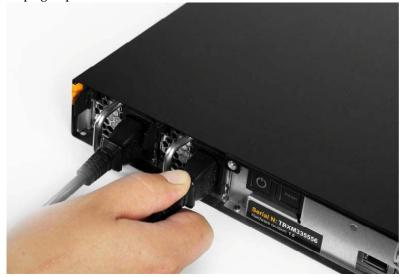
**3.** Holding the lever of the power module with your index finger, push the side tab to the right and slide out the unit from the appliance.
