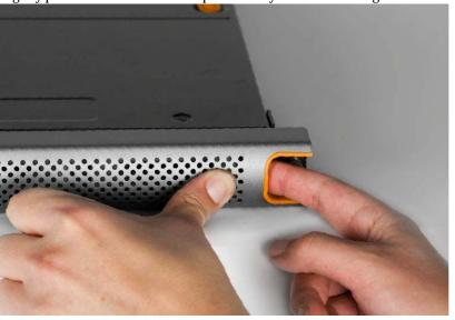
To remove the bezel, with your index finger push inward the release latches at each side of the bezel and gently pull it away from the front panel:
