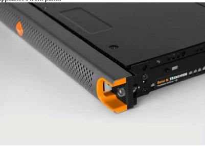
**2.** Using your index finger, push inward the release latch at each side of the bezel and slightly push the bezel to the front panel until you hear a clicking sound.
