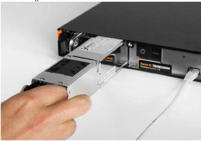
**Tip:** To check that the power module is properly installed, try to pull it out without pressing the side tab. If the power module can be pulled out, repeat the step again.
