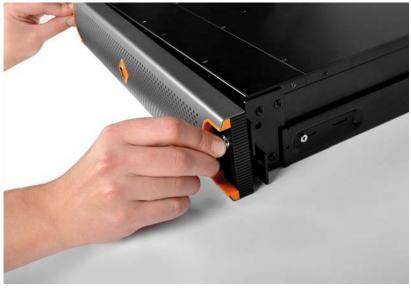
**2.** Gently pull away the bezel from the front panel of the appliance.
