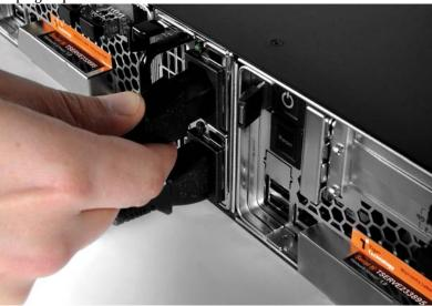
**3.** Press the tab of the module to release it and holding the lever, slide it out of the appliance.
