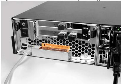
**6.** Plug other end of the network cable in the port of the Ethernet switch that interconnects computers on the network.
