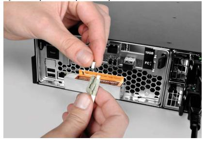
3. Plug one end of the fiber-optic cable into the SFP socket of the FC port.
