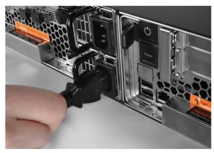
**2.** Connect the power cord to the power outlet.
