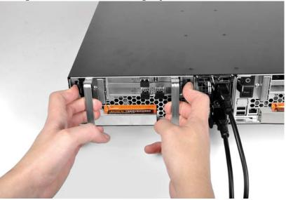
${\bf 5.}$  While pressing the tabs, pull the node by the levers and gently slide it out the appliance. I
