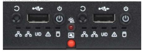
• System reset button and system power button.
