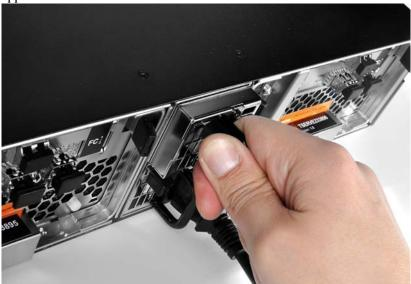
**4.** Insert the new power module until it makes full contact with the enclosure and you hear a clicking sound.
